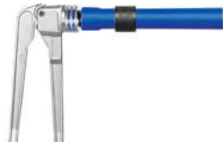
2- Expand the pipe end
